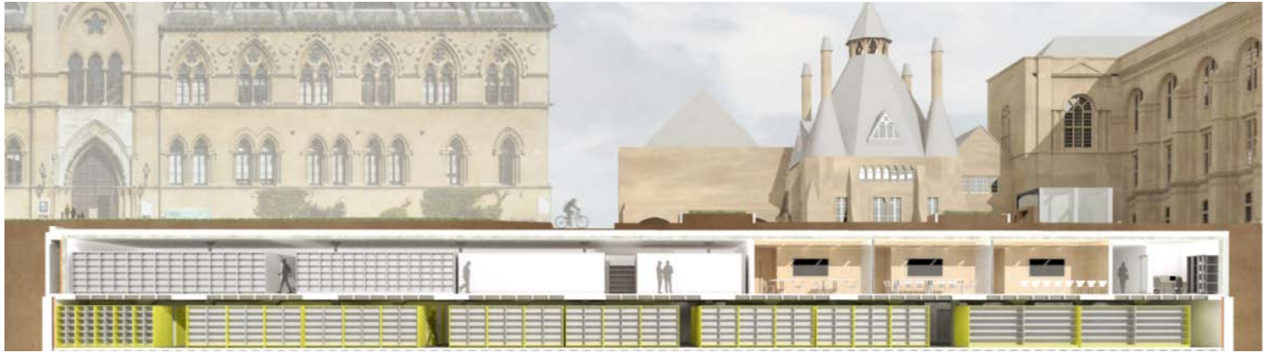
Fig. 1. A diagram showing the location and design of the CTRC. Lift access is through the cube on the right.
