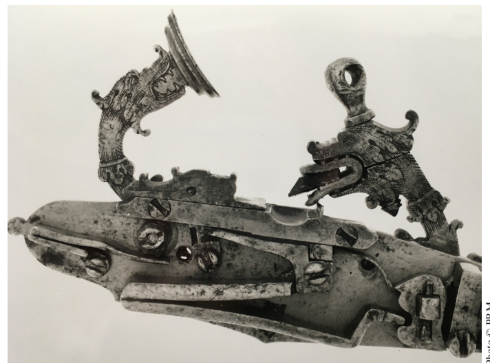
The lock of a snaphaunce pistol; Italian (Brescia), ca. 1645-50. Photo taken from the other side.
